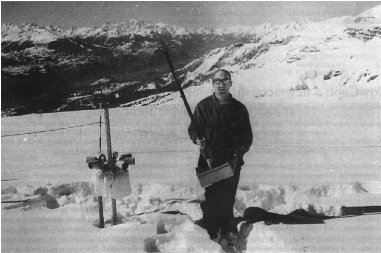
Fig. 1. The Driftometer catches blown snow particles into a collector through a tube by the combined effects of filter and pressure fall. Weighing the collector directly gives a snowdrift index.
