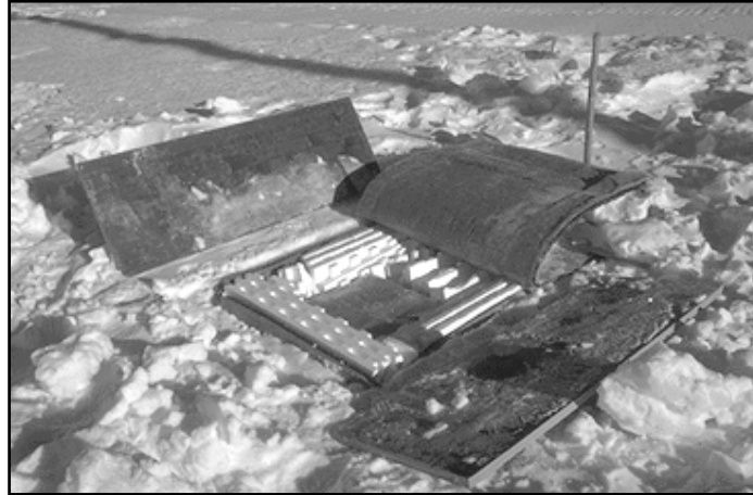
Fig. 4: Special infrasound microphones ECHO, installed under the snow cover
